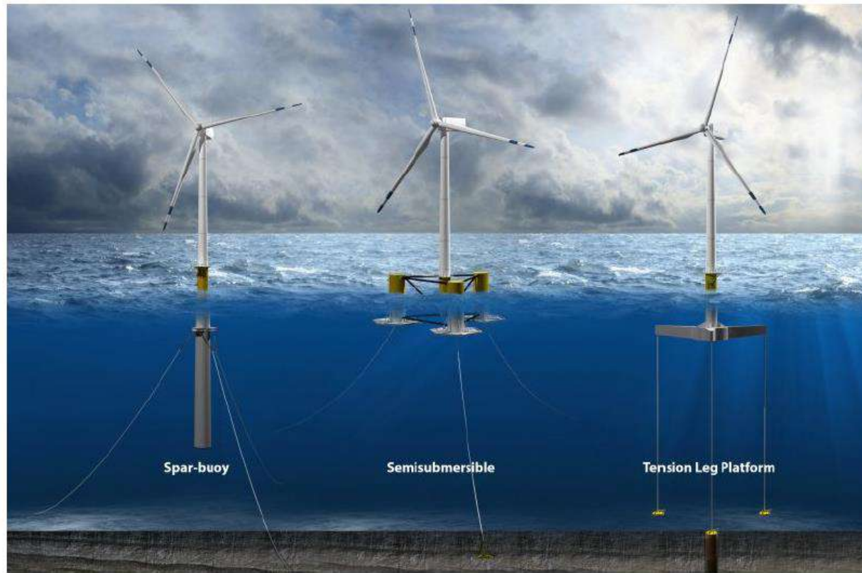
Figure 2.5: The three floater foundation concepts. Spar-buoy (Spar), Semi-submersible (Semi-Sub) and Tension Leg Platform (TLP) [22]
