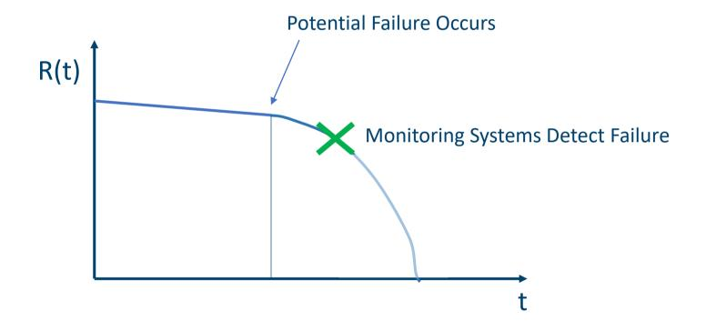
• Monitoring systems may not detect all the possible failure modes....
