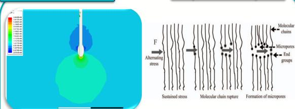
Electrical field is greatly distorted and concentrated at the tip of the water tree. Generates alternating stress acting on polymer chains
