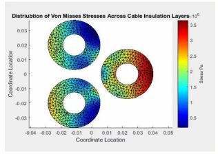
Combining the FEA and the dynamic model can produce a time history of stresses of any cable component., in any environment.
