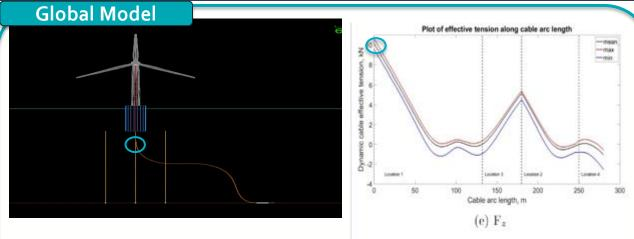
A global dynamic model can be built to show where along the cables length, the environmental forces will be of greatest concern.
